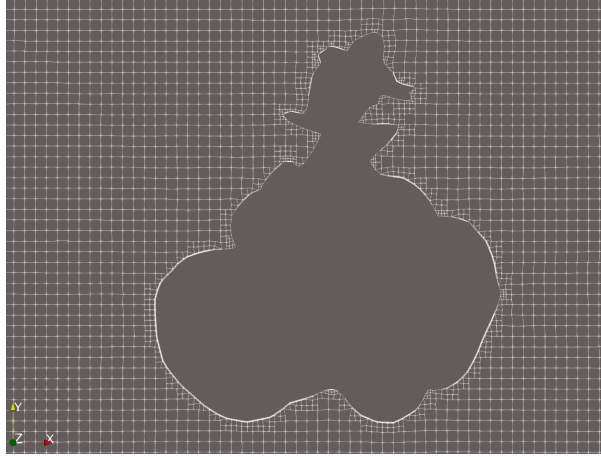
Figure 5: Highlight of the computational mesh around the 2D car profile
